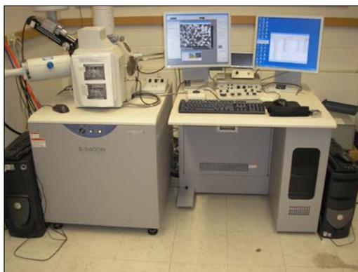
In addition, our SEM can operate in **variable pressure** mode allowing samples to be viewed under minimal vacuum. This feature allows samples that would be compromised by beam energy or vacuum to be imaged and analyzed without any carbon or heavy metal coatings required. Our SEM can view:
